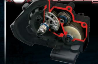
Torque-Control® Slipper Clutch
